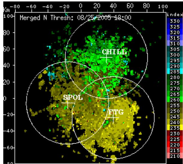
**Fig. 3.** Mosaic of refractivity (N) data from CHILL, S-POL and the NEXRAD FTG radars on 25 August 2005 at 18:00 UTC. Rings represent 50 km range from the radars. High N values represent regions of higher moisture.
