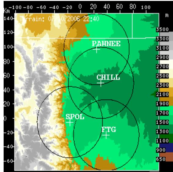
**Fig. 2.** Topographic map of NE Colorado. The rings represent the 50 km range from each radar and approximate coverage of refractivity data during REFRACTT.
