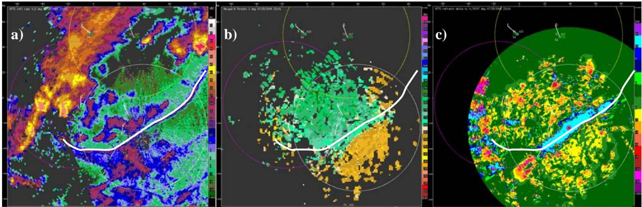
**Fig. 4.** Gust front passage to the south of the Denver NEXRAD FTG radar (white contour) on 25 July 2005. a) reflectivity, b) refractivity, c) delta-N.
