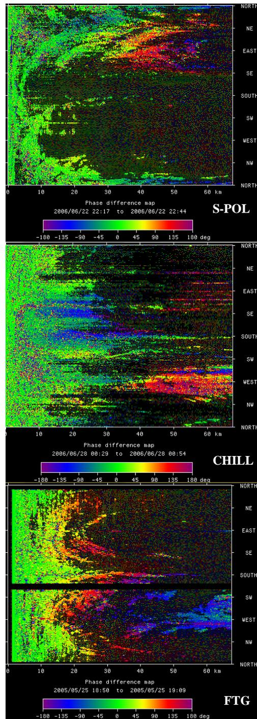
**Fig. 1.** Examples of B-scan phase difference plots used to identify good reference refractivity datasets. Range from radar is along the horizontal axis; azimuthal direction is along the vertical axis. S-POL and CHILL plots are from 22 June 2006. The FTG plot is from 25 May 2005.
