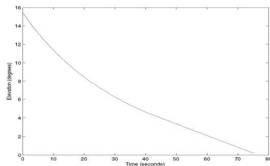
**Fig. 2.** The elevation scan-rate is elevation dependent. The slower scan-rate at low-elevation leads to better detection of weak signals at low altitude and long range.
