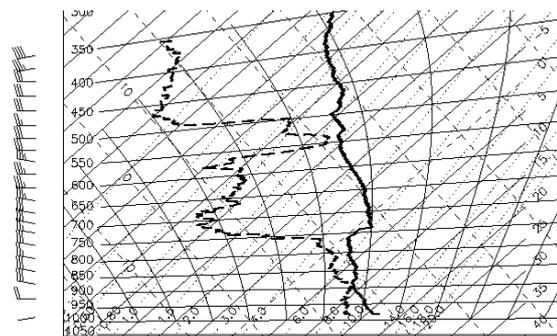
**Fig. 1.** Tephigram for the radiosonde launched from Bath at 1100 UTC (around 60 km from Chilbolton and less than an hour from when the data shown in Fig. 3 was collected).
