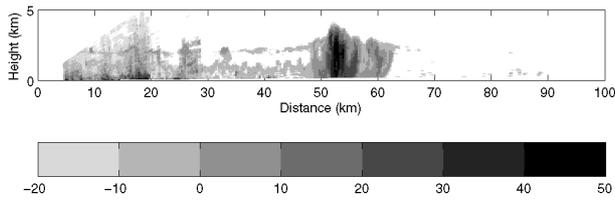
**Fig. 3.** A range-height indicator (RHI) of radar reflectivity showing clear-air echo from the inversion at the top of the boundary layer (e.g. at a height of between 2 and 2.5 km at ranges between 10 and 50 km)
