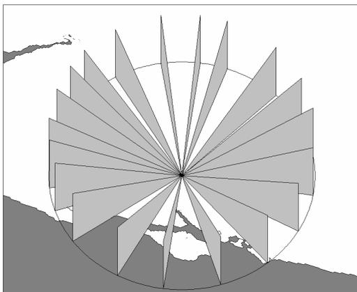
**Fig. 4.** The radar scan sequence comprises 20 RHIs 18 degrees in azimuth apart.
