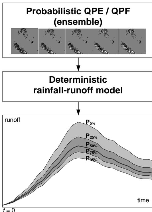
**Fig. 5.** Ensemble of probabilistic precipitation fields as input to rainfall-runoff model and resulting ensemble of hydrographs.
