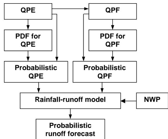
Fig. 1. Scheme of the probabilistic hydrological forecasting.
