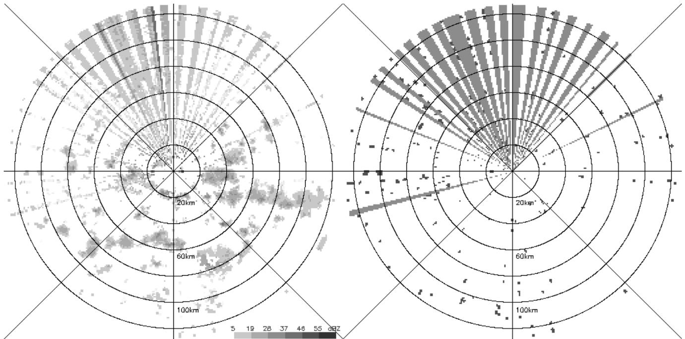
**Fig. 1.** Radar image from 31 May 2006 7:50 UTC at the radar station Munich (left) and the corresponding quality information (right)
