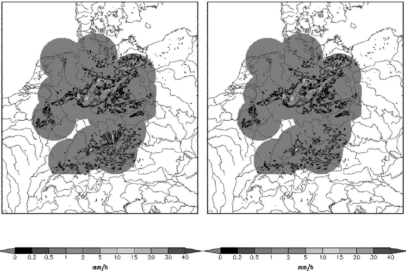
**Fig. 2.** Radar composit from 31 May 2006 at 7:50 UTC using the maximum method (left) and the quality information (right) for assigning pixel values in the overlapping areas. For the radar stations Rostock (in northeast Germany) and Frankfurt (in southwest Germany) no radar data was available at this time.
