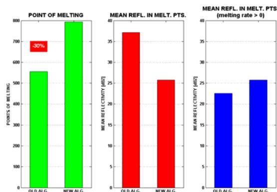
**Fig. 5.** Some statistics about the results retrieved using the two algorithm. NEW\_ALG detects a major number of melting points (i.e. points in which a solid hydrometeors is melting, green bars) while the mean reflectivity of the brightband is minor respect of the one computed with OLD\_ALG (red and blue bars).
