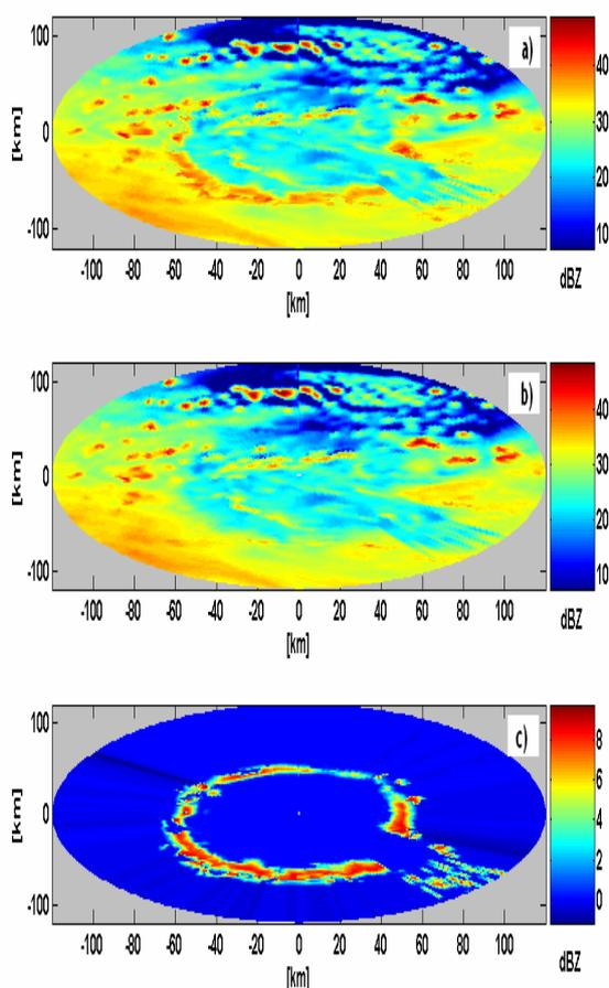
**Fig. 6.** Panel a) shows the PPI plot (performed at  $0.5^\circ$  elevation) obtained by applying NEW\_ALG, panel b) the PPI with no brightband detection algorithm, panel c) displays the difference between the two: the positive difference shows the overestimation due to the melting of solid hydrometeors.
