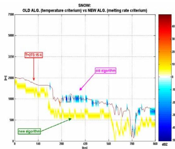
**Fig. 4.** The comparison between the different algorithms: the yellow layer points the re-location of the brightband due to the use of NEW\_ALG.
