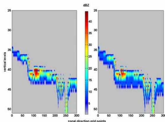
**Fig. 3.** The brightband detected with the OLD\_ALG (on the left) and the NEW\_ALG on the right, the representation seems to be quite similar even if a downward shift of the brightband can be noticed with the NEW\_ALG.
