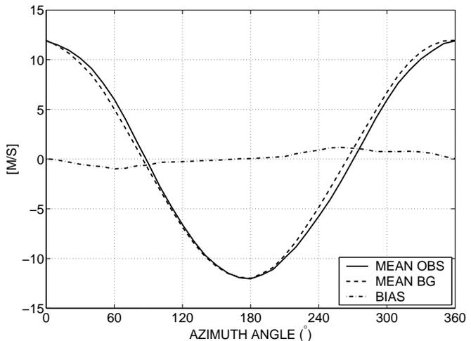
**Fig. 3.** The mean observed radial wind speed (solid line), the mean background radial wind speed (dashed line) and their difference (bias) (dash-dotted line) as a function of azimuth angle.
