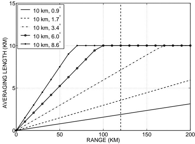
**Fig. 4.** Schematic illustration about the averaging lengths applied in the SO generation at different measurement ranges.
