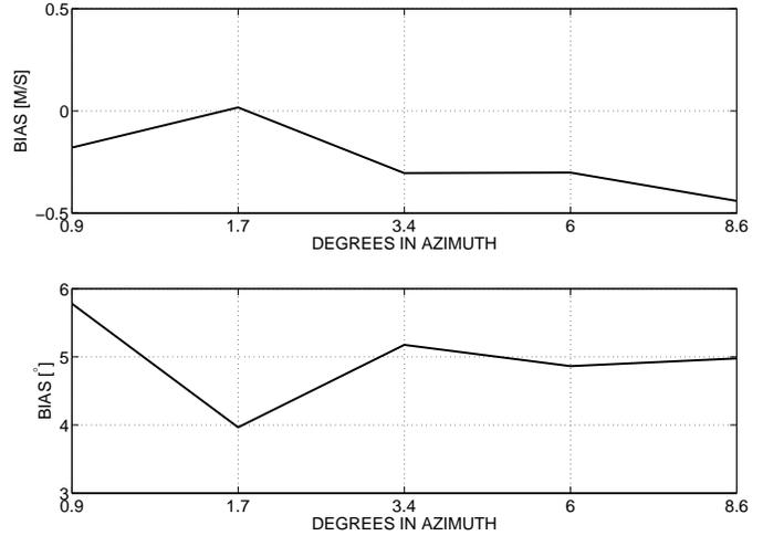
**Fig. 5.** Bias for wind speed (upper panel) and for wind direction (lower panel) shown as a function of SO resolution in azimuth.
