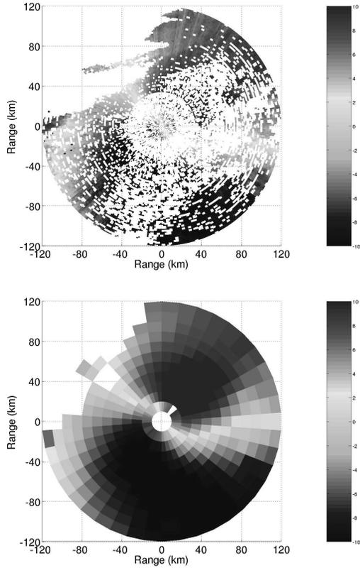
**Fig. 1.** An example of the Doppler radar radial wind data (upper panel) and SOs generated with spatial averaging (lower panel).
