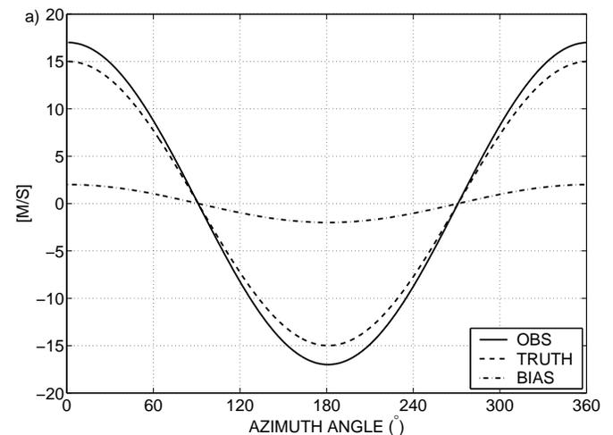
**Fig. 2.** An example of the azimuthal behaviour of radar radial wind bias. Observed wind is 17 m/s from the South (solid line) and true wind is 15 m/s from the South (dashed line). Bias is shown with the dash-dotted line.
