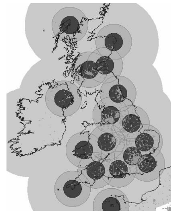
Fig. 2. Met Office radar network. Circles denote resolution of coverage – inner 1km, middle 2km, outer 5km.
