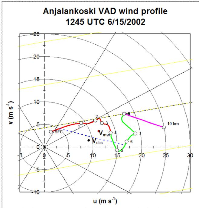
**Fig. 1** A hodograph derived from a velocity wind profile derived from the Anjalankoski radar just to the north of the supercell track. The observed storm motion is plotted as  $V_{obs}$ ,  $V_{mw}$  is the mean 0-6 km wind.
