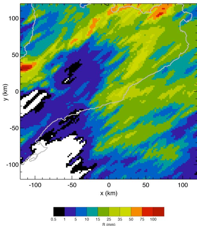
Fig 5. – Comparison of accumulated rainfall by radar by means non-optimized processing and using the system of corrections included in the EHIMI tool.
