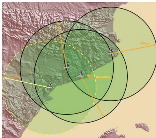
Fig 4. - C band Radar network of the SMC, three radars operate at present moment and a fourth is foreseen for 2007 (dotted).
