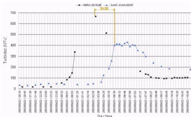
Fig 3. - Example of an event with contamination by turbidity.
