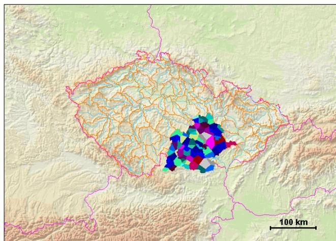
Fig. 3. Thiessens polygons used for areal representation of the rainfall measured by raingauges. The radar and merged estimates in 1x1 km grid are also used for the calculation of the mean areal rainfall for each polygon.
