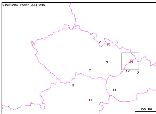
Fig. 2. The square for which the maximum value are “representative”. After the first maximum in the domain is found, then the area around (the square 80x80 km) is blanked and the following less extreme is being searched.
