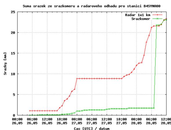
Fig. 3. Example of the comparison of raingauge measurement (lower curve) and collocated radar-based QPE indicating an error of tipping bucket raingauge.
