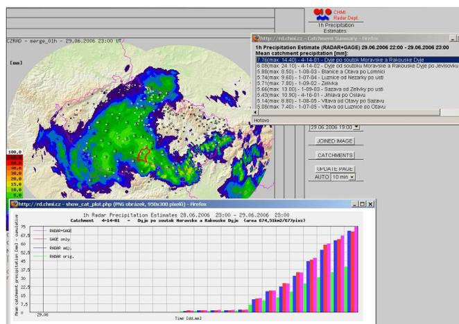
Fig. 1. Example of the combined (merged) QPE in the application JSPrecipView, along with the rainfall accumulation at a predefined catchment that can be chosen by the user. The accumulations are computed for all the types of the precipitation estimate. The tiny squares on the map indicate the raingauge locations.
