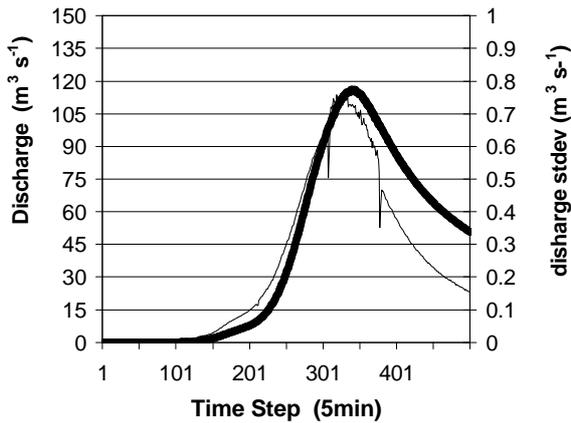
Fig 3 : Mean hydrograph output (bold line) and hydrograph standard deviation (thin line) obtained from the 1000 Monte Carlo simulations
