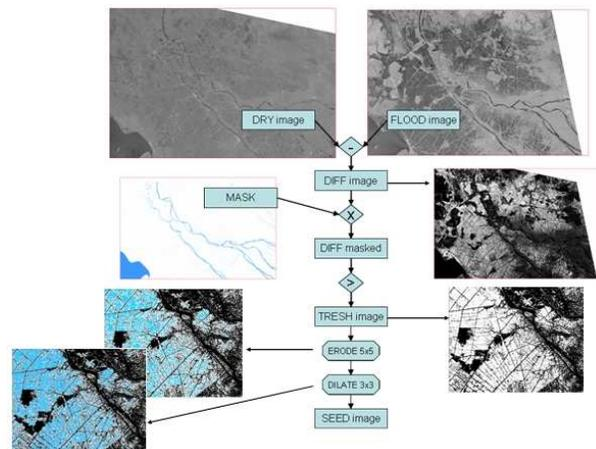
Fig. 3. First steps in the automatic flood recognition.
