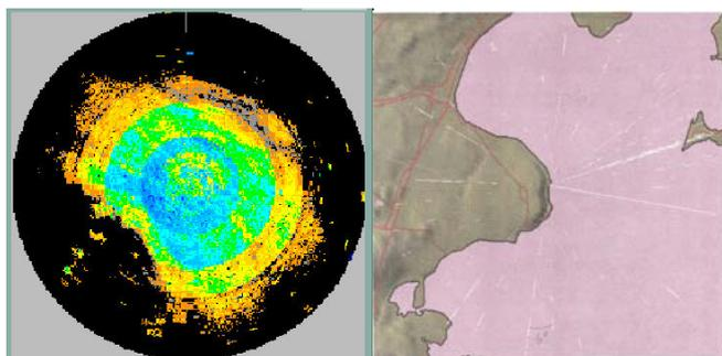
**Fig. 2.** Display of artificial ring structure (left) and the radial streaks (right) caused by external interference at Stevns from 26<sup>th</sup> February 2002.
