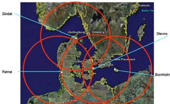
**Fig. 1.** The Danish weather radar network showing the location of the four radars together with the 240 km maximum range.
