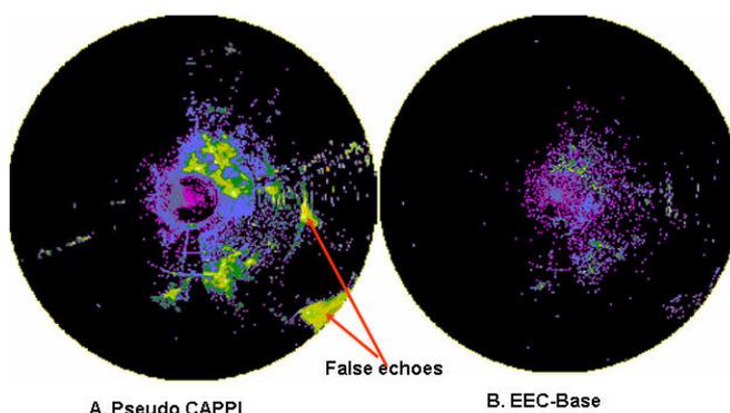
**Fig. 3a.** Display of false echoes (sea clutter) in the pseudo CAPPI and the EEC BASE products by the radar at Stevns 4<sup>th</sup> September, 2004.
