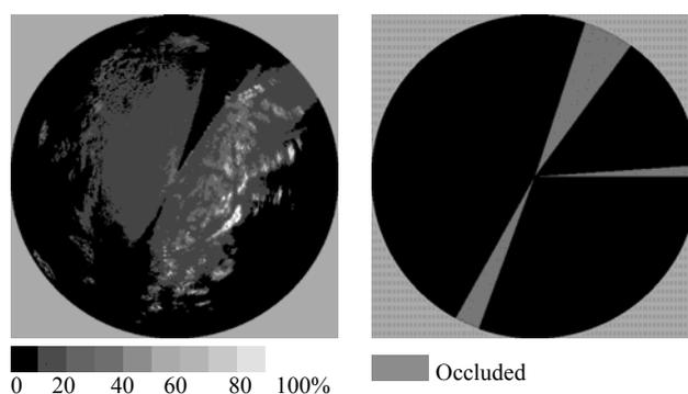
**Fig 4** (a) Probability of detection (b) diagnosis of occultation for the radar at La Dole, Switzerland,
