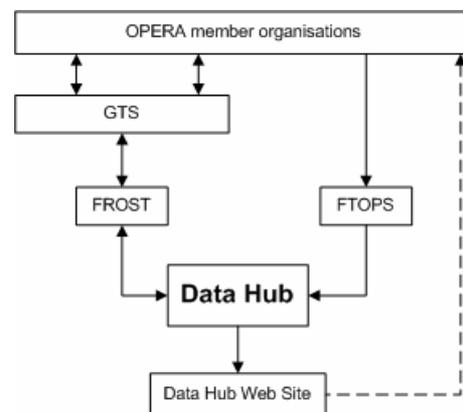
Fig. 2. Diagram of system components and data flows associated with the Data Hub. FROST and FTOPS are the UK Met Office message switching and ftp server systems respectively. The dashed line indicates latest product download via the Data Hub web site.
