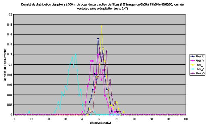
**Fig. 2.** Measured impacts of wind farms on meteorological radars
