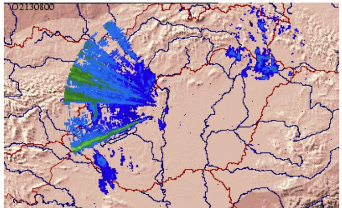
Fig. 1. Interference from RLAN 5 GHz to Budapest radar
