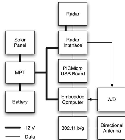
**Fig. 3.** OTG prototype block diagram
