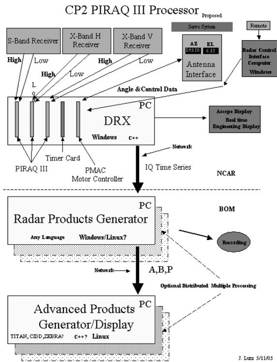
**Fig. 3** Simplified schematic of updated CP2 signal processor, control, product generator and display systems.
