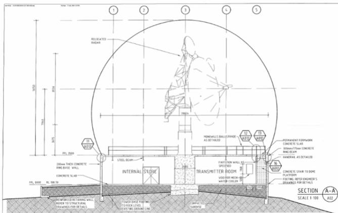
**Fig. 4.** CP2 site infrastructure. Antenna and pedestal within an inflated radome are mounted over housing for office, storage and transceiver.
