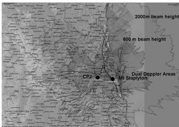
**Fig. 1.** Topography, surrounding environment and range where the CP2 beam height (m) intersects various levels. Dual Doppler lobes available using the Mt Staplyton Doppler radar and CP2 are indicated.
