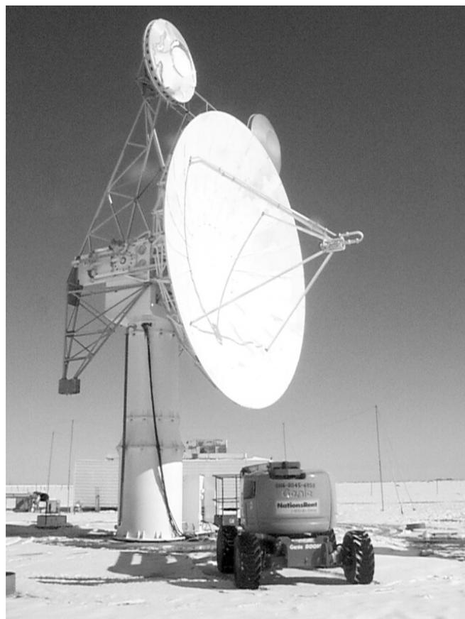
**Fig. 2.** CP2 pedestal and antenna during testing at Boulder. Two X-Band cassegrain paraboloids are located above the primary centre fed S-Band paraboloid dish.
