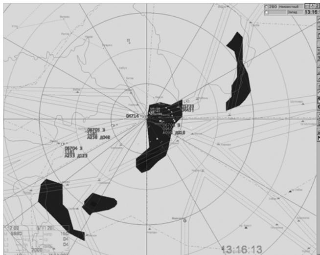
Fig. 2. Meteorological radar data on the screen of air traffic controllers.
