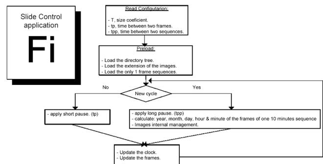
Fig. 3. Slide control application scheme.
