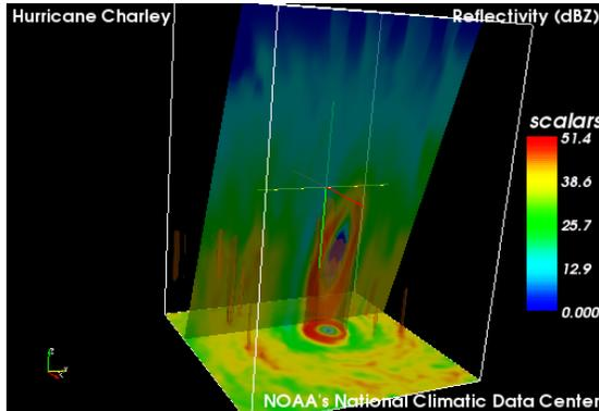
**Fig 8. VTK multimedia screenshot using ParaView software displaying data exported using Radar Data Exporter tool**
