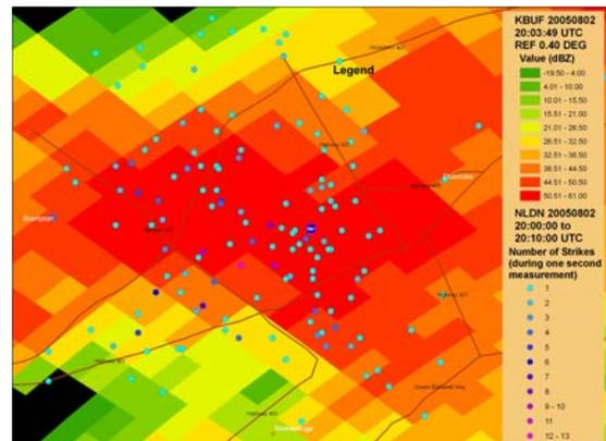
Fig. 7. Radar data and lightning data exported to SHP file and displayed in ESRI GIS software for Toronto A.P. August 2, 2005 event
