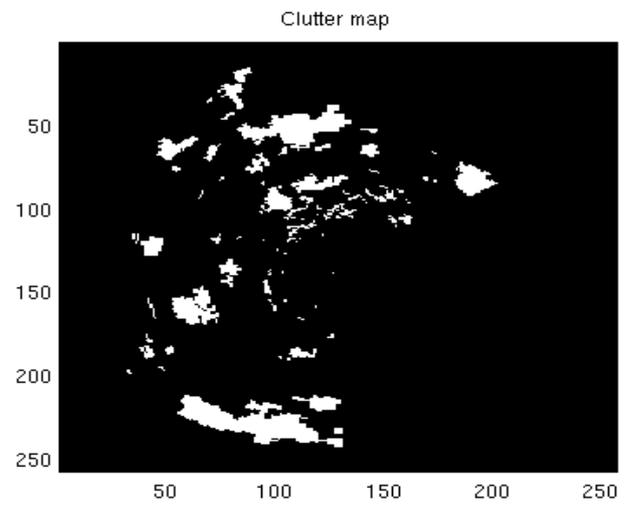
**Fig. 1.** Illustration of clutterremoval. a) is the cleaned map, b) the map before processing and c) is the unprocessed map 10 timesteps earlier. Finally d) is the cluttermap created for this event. The four '+' indicate where the raingauges were located.
