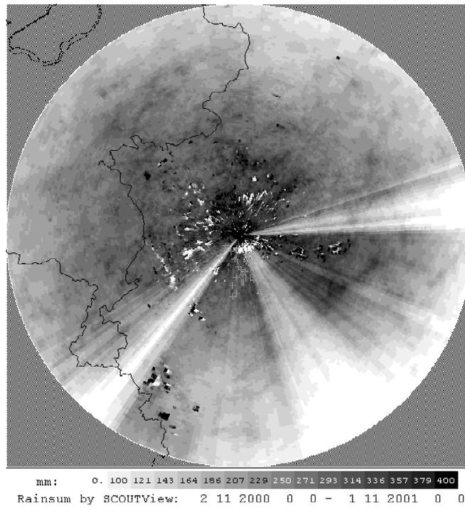
Fig. 1. Sum of one year of uncorrected and non-adjusted radar measurements
