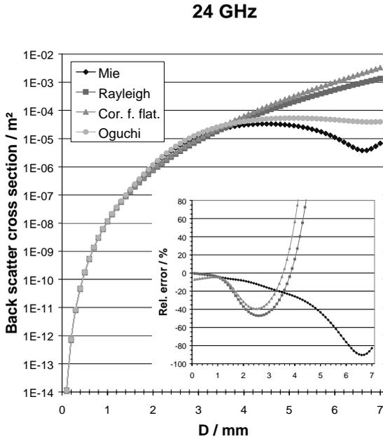
**Fig. 2.** Comparison of backscatter cross section versus drop diameter at 24 GHz calculated from the different scattering theories. The correction of the Rayleigh backscatter cross section for drop flattening is calculated according to Eq. (6). The small inset shows the relative error with respect to the backscatter cross section according to Oguchi, as defined by Eq. (7).
