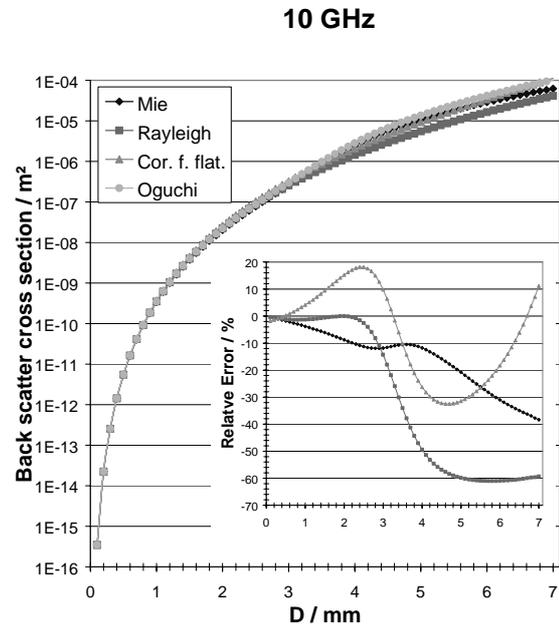
**Fig. 1.** Comparison of backscatter cross section versus drop diameter at 10 GHz calculated from the different scattering theories. The correction of the Rayleigh backscatter cross section for drop flattening is calculated according to Eq. (6). The small inset shows the relative error with respect to the backscatter cross section according to Oguchi, as defined by Eq. (7).
