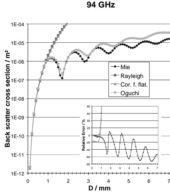
**Fig. 3.** Comparison of backscatter cross section versus drop diameter at 94 GHz calculated from the different scattering theories. The correction of the Rayleigh backscatter cross section for drop flattening is calculated according to Eq. (6). The small inset shows the relative error with respect to the backscatter cross section according to Oguchi, as defined by Eq. (7).
