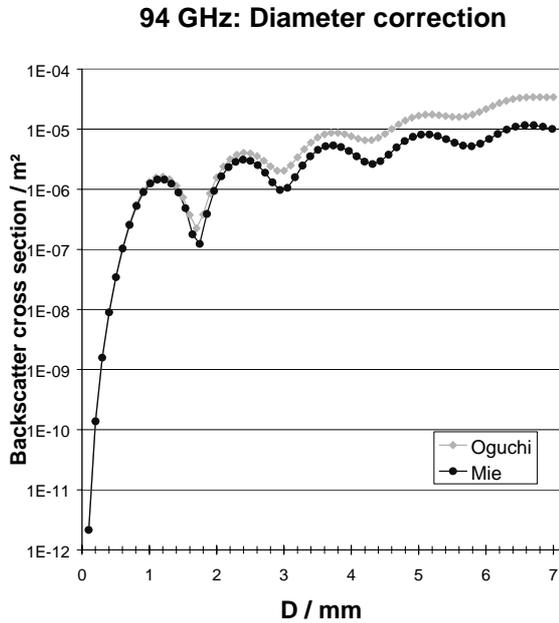
**Fig. 4.** Comparison of backscatter cross section versus drop diameter at 94 GHz calculated by Oguchi and Mie code, respectively. For the Mie calculation, the original diameter has been corrected by multiplying by  $\beta^{1/6}$  (see Eqs. (1) and (8)).
