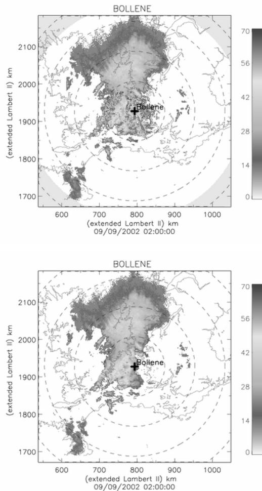
**Fig. 1.** Radar reflectivity PPI corresponding to an elevation angle of  $0.8^\circ$  the 9 September 2002, 2h: uncorrected data (top) and corrected data thanks to the adaptive ground clutter identification and interpolation (bottom).
