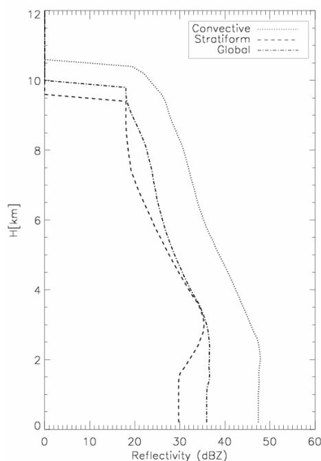
**Fig. 3.** VPR corresponding to global, convective and stratiform rain type for the same date as in Fig. 1.
