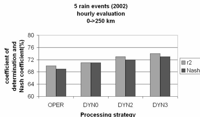
**Fig. 4.** Evaluation of the OPER and DYN processing strategies: Coefficient of determination and Nash criteria at the hourly time step for the whole of the five rain events.
