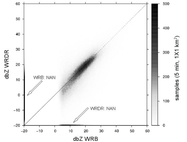
**Fig.2.** Comparison of radar reflectivity between WRDR and the DWD weather radar Berlin (WRB).
