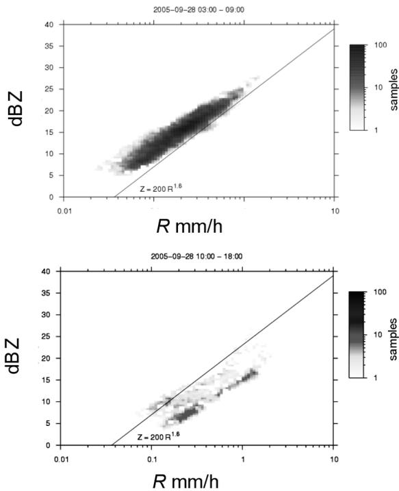
**Fig.3.**  $Z$  versus rain rate  $RR$ . The solid lines represent a standard  $R(Z)$ -relation. Top: 6-hour interval with larger drops. Bottom: Subsequent 8-hour interval with smaller drops.
