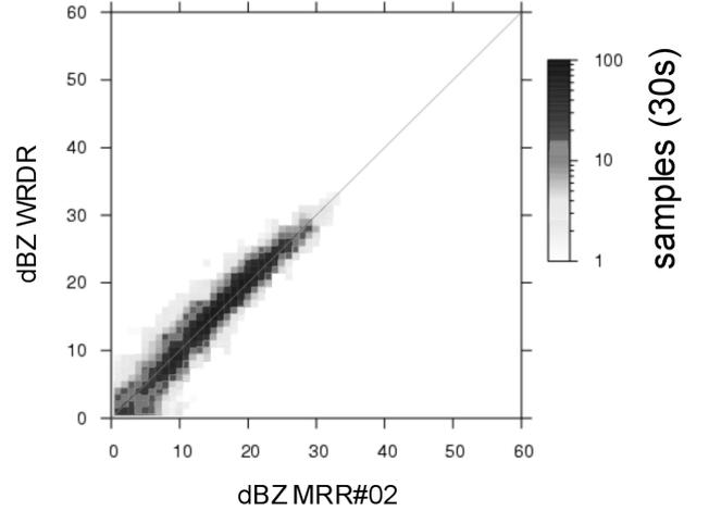
**Fig.1.** Comparison of radar reflectivity between WRDR and MRR#02
