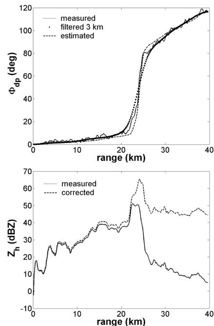
Fig. 1. An example of severe attenuation and correction of radar horizontal reflectivity  $Z_h$ .
