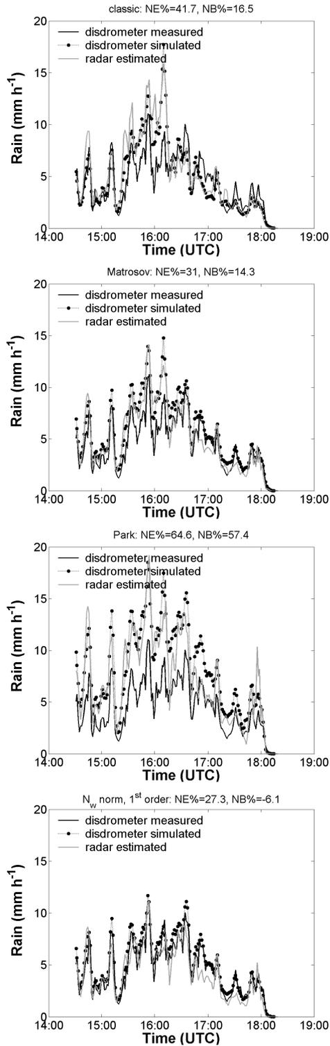
**Fig. 4.** Time series of disdrometer measured rainfall and estimators from disdrometer simulated and radar measured  $Z_h$ ,  $K_{dp}$ , and  $Z_{dr}$  during a stratiform like rain event (17/11/2005).
