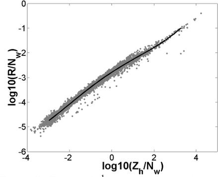
**Fig. 3.** Rainfall  $R$  ( $\text{mm h}^{-1}$ ) and simulated reflectivity  $Z_h$  ( $\text{mm}^6 \text{m}^{-3}$ ) normalized by the measured intercept parameter  $N_w$  ( $\text{mm}^{-1} \text{m}^{-3}$ ) for the full disdrometer dataset. A 4<sup>th</sup> order polynomial is fitted to the data.
