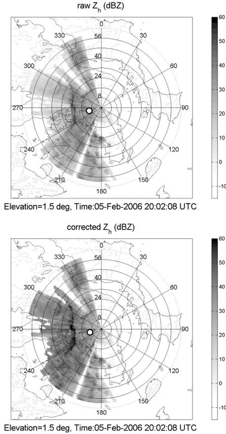
**Fig. 2.** PPI images of  $Z_h$  before and after attenuation correction corresponding to Fig. 1. The shoreline and disdrometer site (white dot) are also shown.
