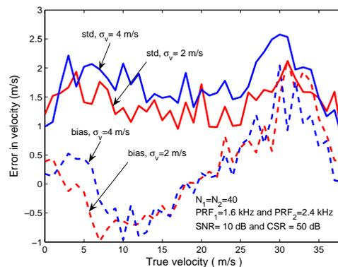
Fig. 6. Bias and standard deviation of velocity after ground clutter filtering for a dual-PRF waveform.
