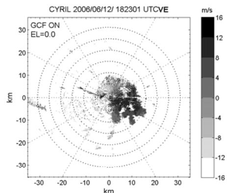
Fig. 5. Velocity after ground clutter filtering.
