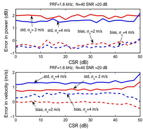
**Fig. 1.** Bias and standard deviation of reflectivity and velocity after ground clutter filtering with PRF=1.6 kHz and N=40.
