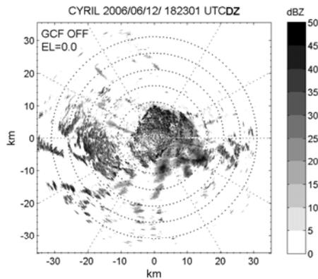
Fig. 2. Reflectivity before ground clutter filtering.
