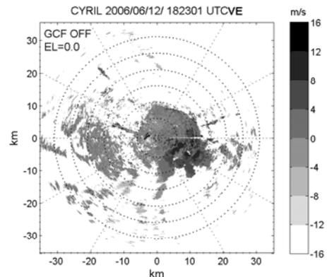
Fig. 4. Velocity before ground clutter filtering.
