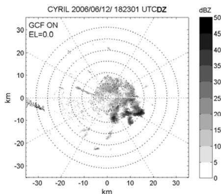
Fig. 3. Reflectivity after ground clutter filtering
