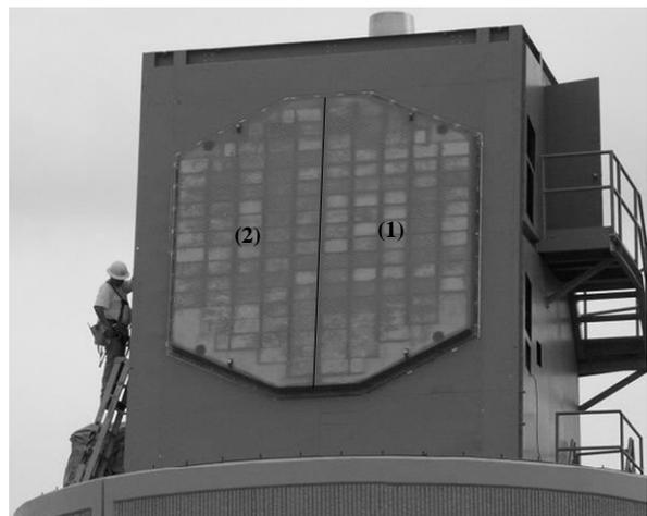
Fig. 1 The NWRT antenna before the installation of an enclosing radome. Marked are the left (1) and right (2) halves of this array.
