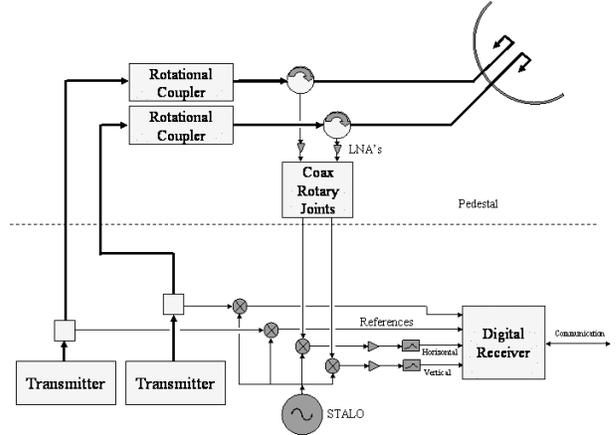
**Fig. 3.** Typical dual transmitter simultaneous dual polarization radar system
