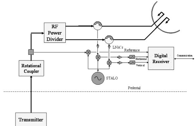
**Fig. 4.** EEC implementation of simultaneous dual polarization radar.
