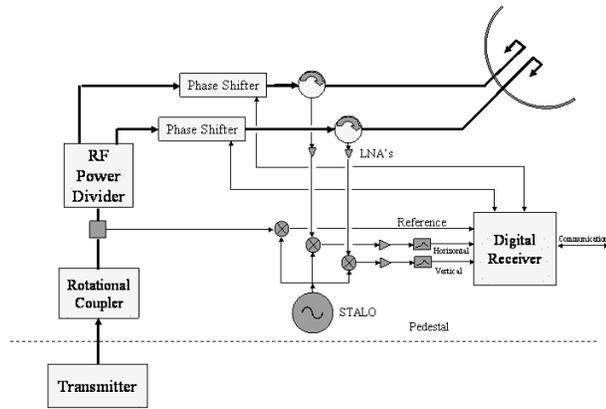
Fig. 6. Block diagram for single transmitter configuration for measuring  $L_{DR}$  simultaneously with the other polarimetric variables
