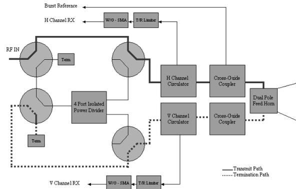
**Fig. 5.** Waveguide network showing switching required with current simultaneous dual polarization radar system measuring  $L_{DR}$ .
