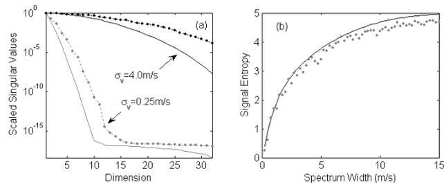
**Fig.1.** Comparison of singular value distributions and entropies: (a) The singular value distribution (scaled with respect to the maximum singular value) for signals with  $\sigma_v$  of 0.25m/s and 4m/s; (b) The signal entropy. The solid lines correspond to theoretical curves, while the dotted lines are based on simulation ( $N=128$  and  $M=32$ ).
