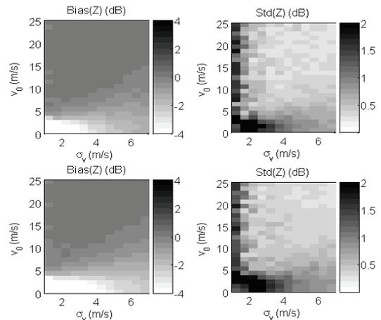
**Fig.4.** Clutter mitigation performance of the adaptive TSVD filter at 40dB CSR (the top row) and 60 dB CSR (the bottom row) based on 100 realizations. The spectrum width and mean velocity of weather signal are given in X- and Y-axis respectively. Clutter has zero mean velocity and  $\sigma_v$  of 0.25m/s. SNR=10dB,  $N=128$ , and  $M=32$ .
