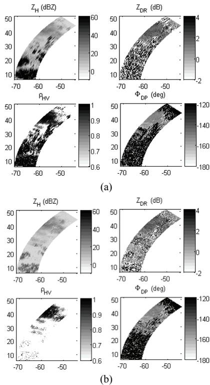
**Fig.3.** PPI plot of dual polarization radar parameters estimated (a) before and (b) after the adaptive TSVD filter. The observations were collected by the CSU-CHILL radar at simultaneous transmission mode on 2145 UTC 24 June 2004. The elevation angle was set at 0.49°, PRF=1000Hz,  $N=128$ , and  $M=32$ .
