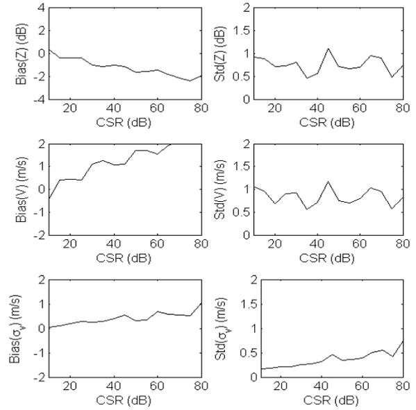
**Fig.2.** Clutter mitigation performance of the adaptive TSVD based on 100 realizations. Clutter is simulated with zero mean velocity and  $\sigma_v$  of 0.25m/s; weather signal is simulated with mean velocity of 5m/s and  $\sigma_v$  of 4m/s; SNR=10dB,  $N=128$ , and  $M=32$ .
