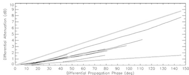
**Fig. 4:** Differential attenuation as a function of the differential phase: one curve per episode (in black); theoretical limits (grey lines).
