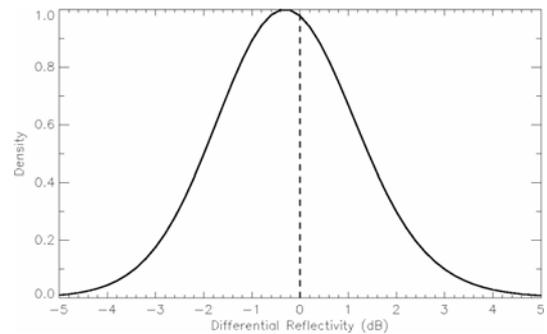
**Fig. 3.**  $Z_{DR}$  calibration diagrams derived from solar radiation collected by the Trappes radar
