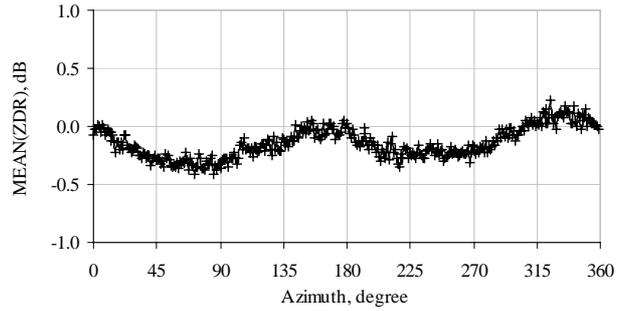
**Fig. 2.**  $Z_{DR}$  calibration diagrams derived from data collected in rain at vertical incidence by the Thurnham radar
