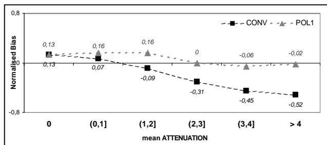
**Fig. 5:** Normalized bias of the ZPHI and conventional rain rate estimator as functions of the mean attenuation over the hour.
