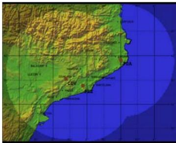
Figure 1. Coverage of the 3-D volumetric radar observations of the Meteorological Service of Catalonia radar network. Radar sites are indicated in red.
