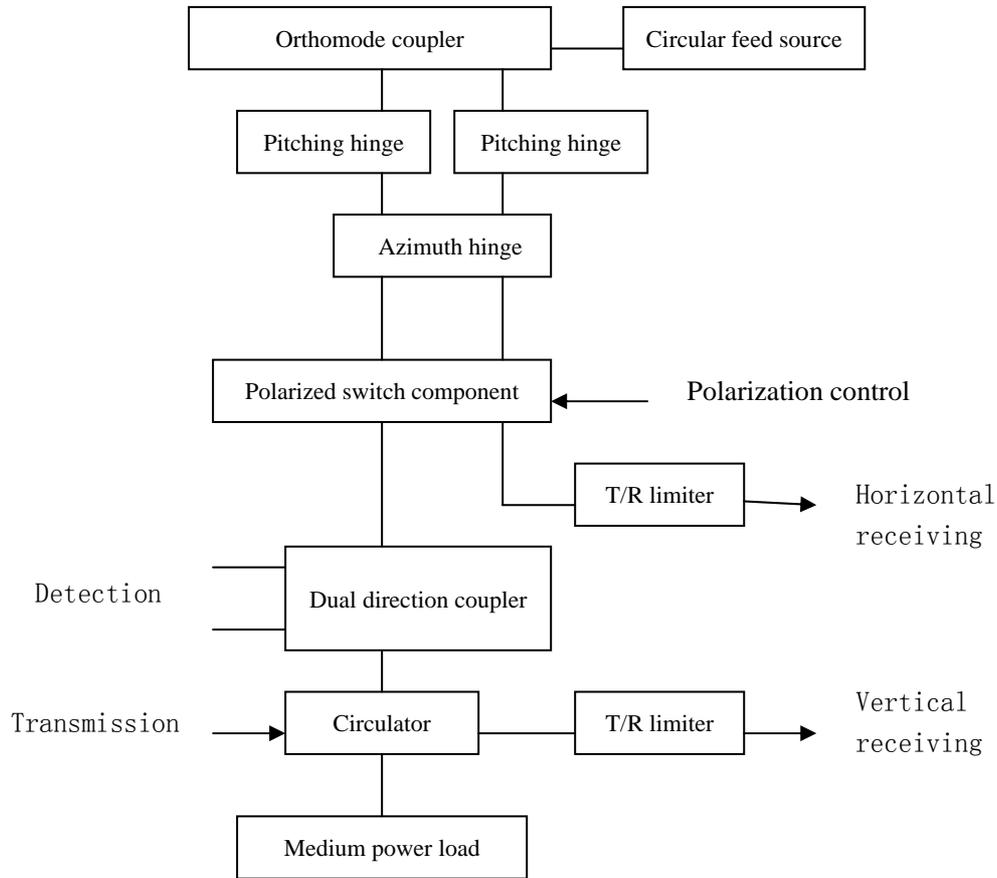
**Fig.1 Block diagram of dual channel system**
