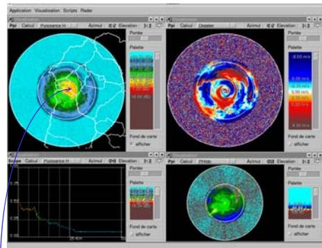
Detection of the bright band at an altitude of 4.1km for the same system as above, a few minutes later.
