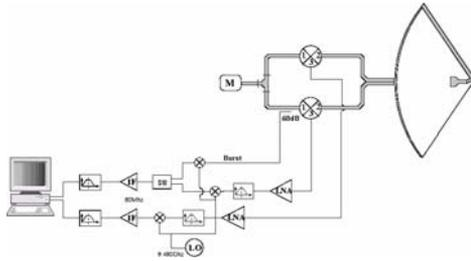
To have a good reception of the small echoes we have chosen a LNA with a strong amplification. In order to achieve a better dynamic and avoid saturation in the first kilometers, we added a 2 step 20 dB attenuator before the LNA. This attenuator works only for short distance.
