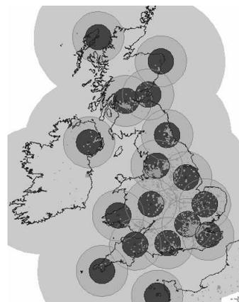
**Fig. 2.** Met Office radar network. Circles denote resolution of coverage – inner 1km, middle 2km, outer 5km.
